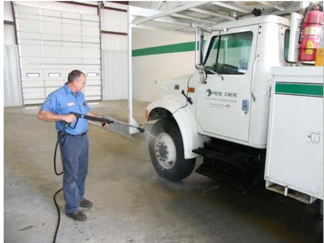
PDEC's Edward Stokes rinses a fleet bucket truck in step one of keeping this unit looking good. The pressure hose is 50-feet long. Addition of a special soapy emulsion is easily attained by turning a small handle on the wand's shaft. The wash bay is 80-feet long and there are two pressure hose/wand combinations, so two full-size trucks may be washed at any time.
